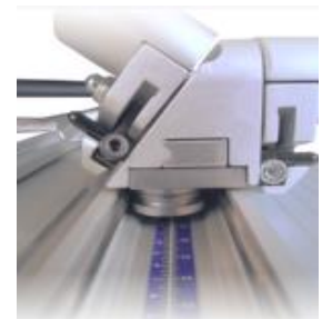
Ultimat sliding gauge and the "start of cut" micro stop
