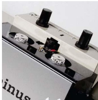
Independent Adjustable Blade Depths on each Head
